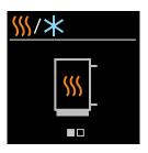
You can select heating or cooling with the buttons + and -. Confirm the selection with the button  $\bullet$
