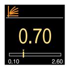
Depending of step 3, you can set steepness of heating or cooling curve. The steepness can be set with the button + and -. Confirm the set steepness with the + button. If you have mistakenly selected the wrong steepness, you can return to selecting the steepness with the + button.
